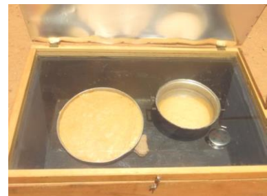
Sunlight has provided the heat that baked these cakes in one hour and twenty minutes.
